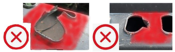
Fig 5. Cracked hook passage holes prohibited for lashing
